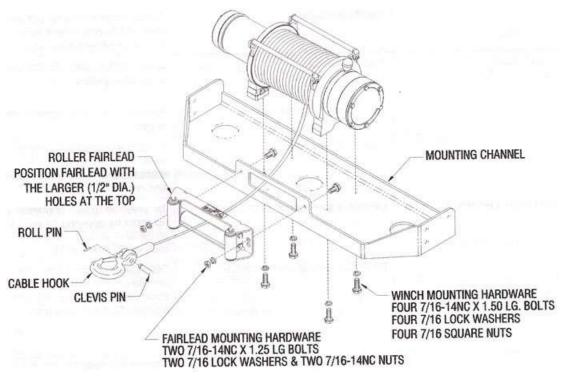
To secure the winch, always use a flat, mounting location with thick enough steel. Always use flat washer, lock washer, long hex head cap screw and so on. Bolt length will be decided by the thickness of mounting location.
